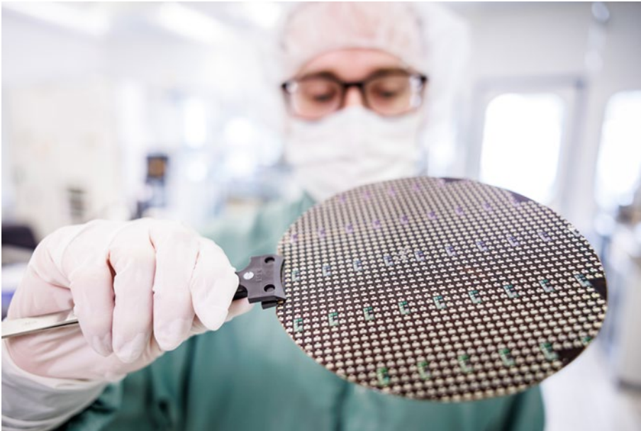
Power devices on a silicon carbide wafer, processed in the in-house cleanroom of Fraunhofer IISB. © Daniel Karmann / Fraunhofer IISB
