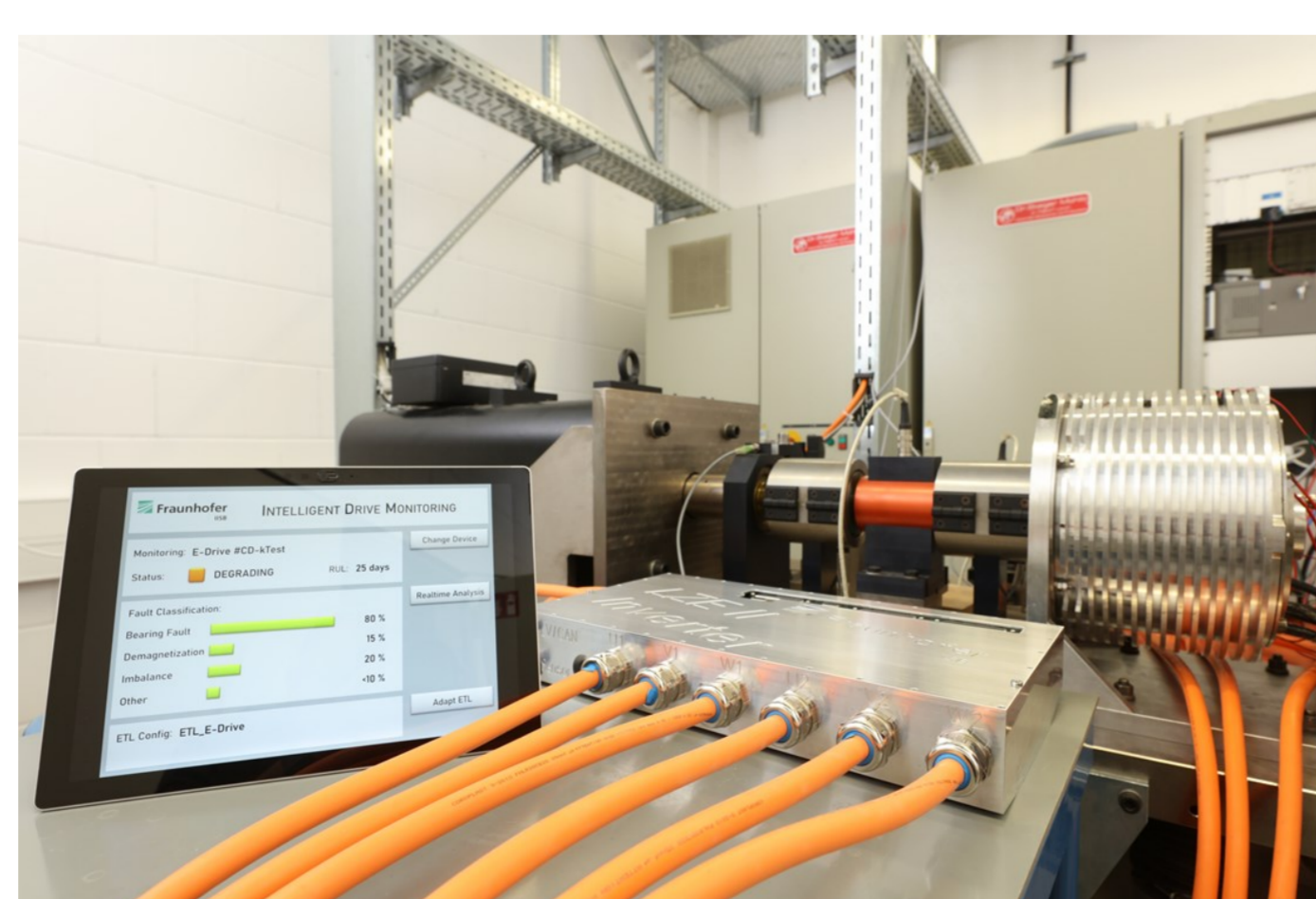
Motor-test bench (© Kurt Fuchs, IISB)
