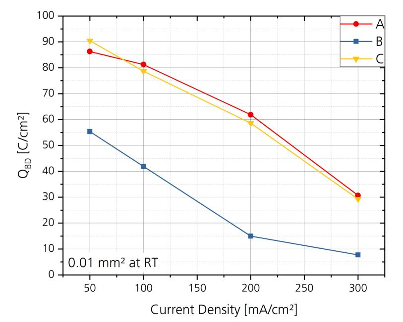
Both CCS-TDDB and Q<sub>BD</sub> extraction at a failure rate of 63 % show identical oxide reliability
