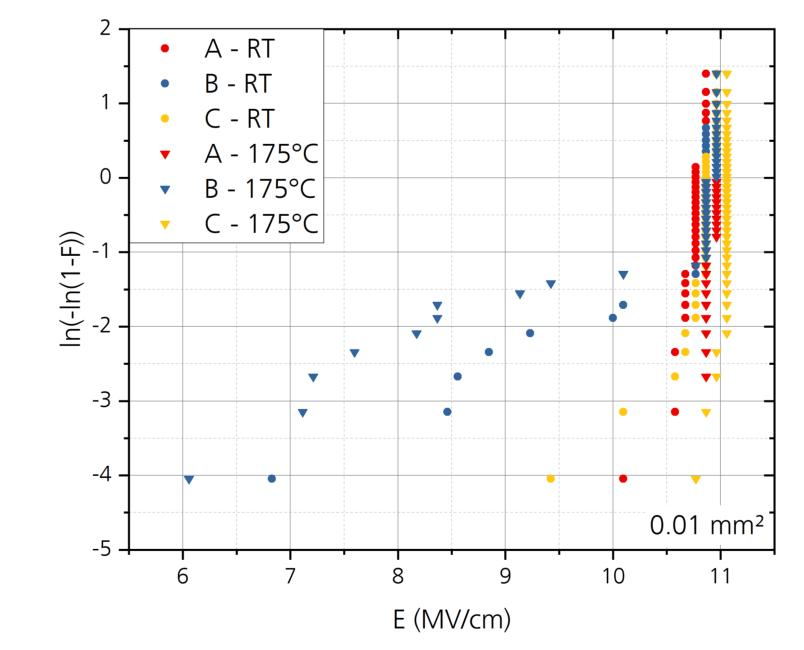
Yield analysis for all sizes and temperatures display no notable differences between standard Weibull plots of TDDB investigations at different temperatures and device sizes show a clear gap in oxide lifetime between RTA and non-RTA processed wafers
