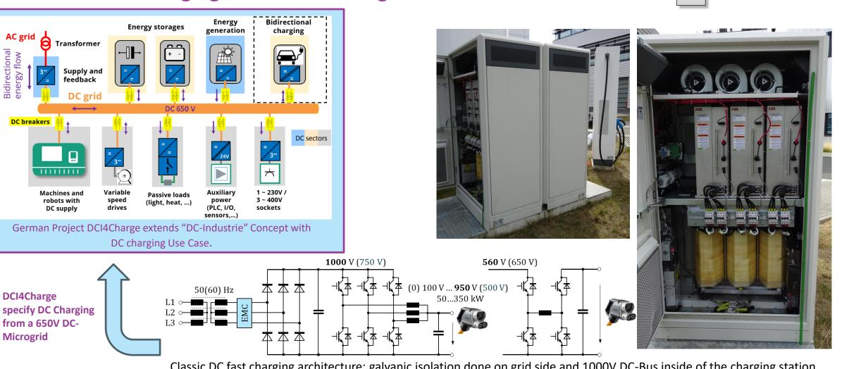
Classic DC fast charging architecture: galvanic isolation done on grid side and 1000V DC-Bus inside of the charging station. This concept only enables one fast DC charger behind the transformer (according to IEC 61851-23).
