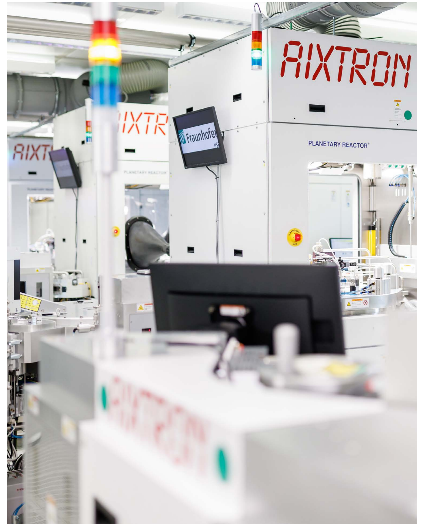
Several Planetary Reactors Are Running in the Joint Lab for Hardware and Process Development with AIXTRON SE, Including the Latest G10-SiC Reactors in 9 x 150 mm and 6 x 200 mm Configurations for Process Tuning and Customer Demonstrations.
