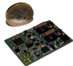
Fig. 1: Intelligent 48V-GaN based primary resonant converter ( P=250W and f>1MHz )
