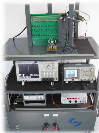
Fig. 4: Low-inductive measurement setup for dynamic device evaluation up to 2000 V, 100 A.
