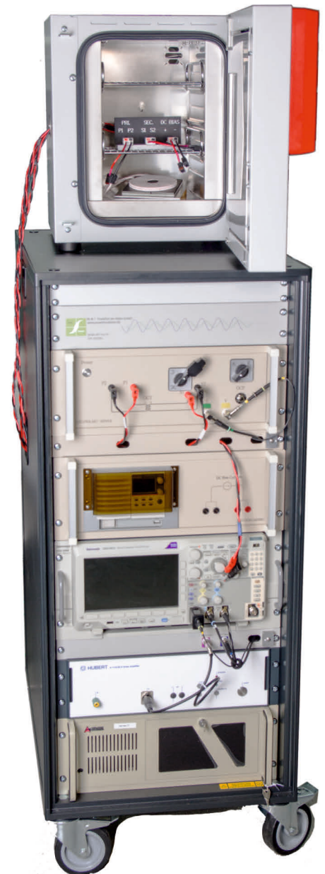
Fig. 4: Test bench for testing inductive components and soft magnetic materials
