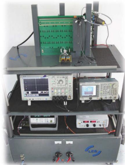
Fig. 4: Low-inductive measurement setup for dynamic device evaluation up to 2000 V, 100 A.
