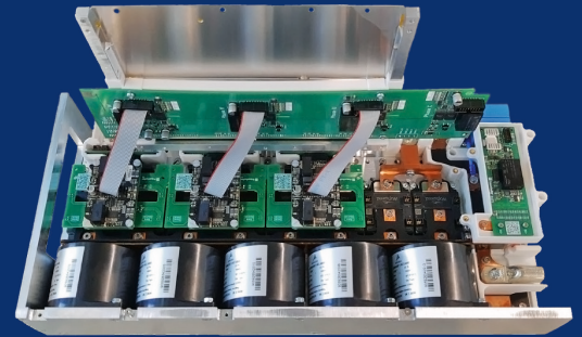
Inside view of the inverter
