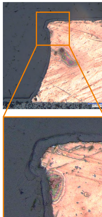
Microscopic images of a parylene coated metallization edge: homogeneous parylene coating with good edge covering © Helena Waldau / Fraunhofer IISB
