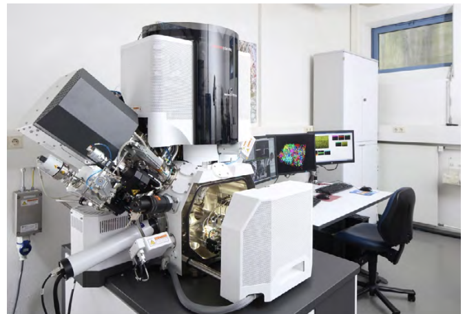
Xe + -Dual beam plasma FIB system at the IISB © Kurt Fuchs / Fraunhofer IISB
