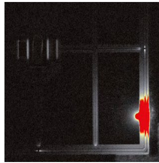
Lock-In-Thermography amplitude of IGBT © Thomas Götz / Fraunhofer IISB
