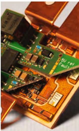
Engineering: vGaN-ready power module with integrated gate driver stage © Elisabeth Iglhaut / Fraunhofer IISB
