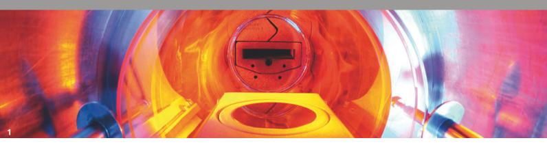
1 View into horizontal hot-wall reactor for SiC homoepitaxy during wafer loading. Image: Kurt Fuchs / Fraunhofer IISB
